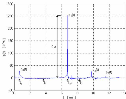
**Figure 1.** Pressure wave radiated by an oscillating spark generated bubble.
