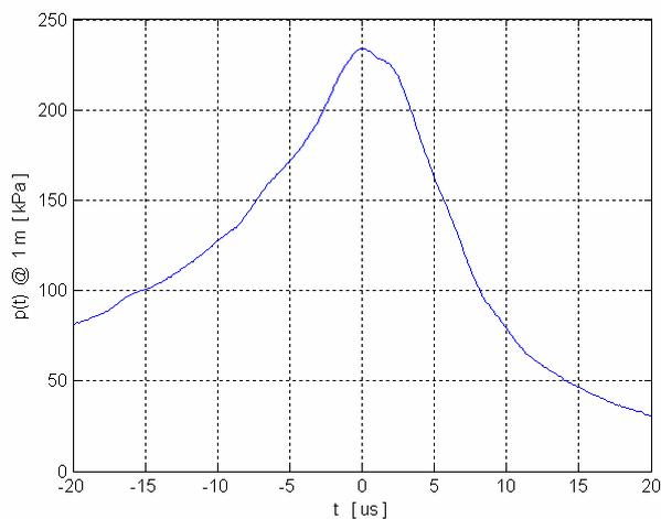
**Figure 3.** Detailed view at the first bubble pulse radiated by a bubble oscillating with a moderate intensity.  $R_{MI} = 44.7 \text{ mm}$ ,  $p_{zpl} = 41.9$ .
