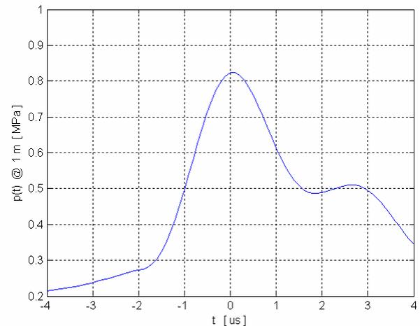
**Figure 4.** Detailed view at the first bubble pulse radiated by a bubble oscillating with a high intensity.  $R_{MI} = 46.6 \text{ mm}$ ,  $p_{zpl} = 141.3$ .
